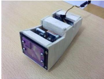
**Fig. 1** Miniature laser rangefinder MRL100 from AERIUS.
